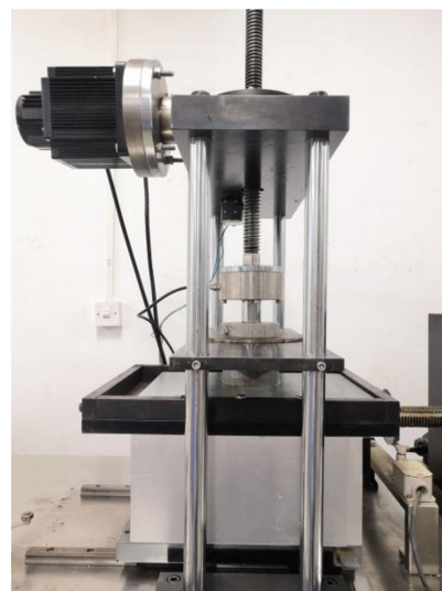
Figure 3. Physical drawing of the direct shear test.
