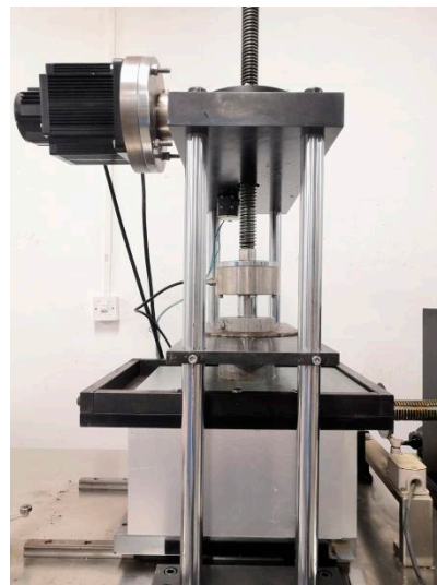
Figure 3. Physical drawing of the direct shear test.
