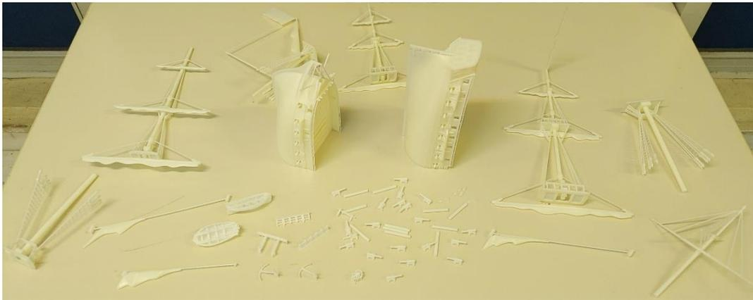
**Figure 22.** Finished products after alcohol rinse and UV cure.
