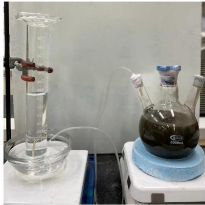
**Figure 2.** Experimental setup of quantification of metallic aluminum in MIBA.
