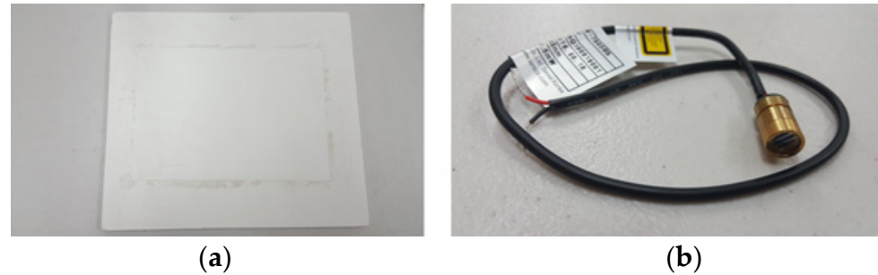
Figure 2. Calibration tool to calibrate the sensor. (a) calibration object; (b) line laser.
