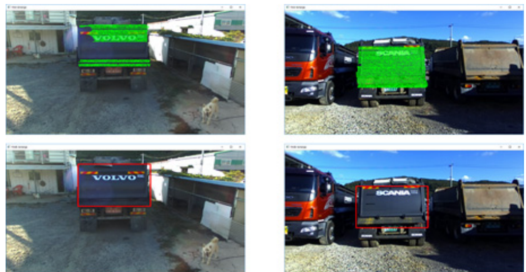
Figure 20. The result of detecting the doors of two commercial dump trucks with LiDAR data. The green point cloud is the point cloud obtained from the stereo camera projected onto the dump truck door plane.
