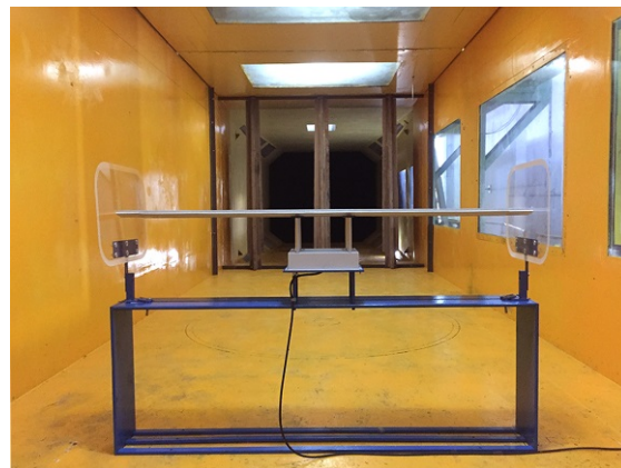
Figure 10. Aerodynamic admittance function identification test.
