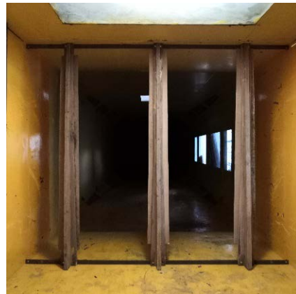
Figure 5. Spire turbulence field installed in XNJD-1 wind tunnel.
