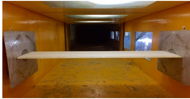
Figure 8. Three-component force test of sectional model.
