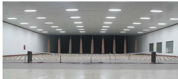
Figure 12. Taut strip model test conducted in XNJD-3 wind tunnel.
