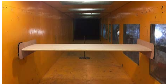
Figure 9. Aerodynamic derivative identification test.
