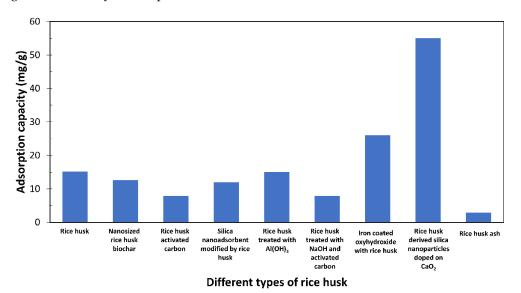
Figure 8. Adsorption capacities by different types of rice husk [78,100,101,104,106–109].
