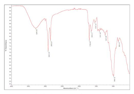
**Figure 6.** FTIR spectra of rice bran (own source) acquired at room temperature by a Nicolet FTIR iS10 spectrometer (Nicolet, Madison, WI, USA) equipped with Smart iTR with diamond plate on Carnaroli rice bran. The waste was dried at 45  $^{\circ}$ C before analysis. Thirty-two scans in the 4000–600 cm<sup>-1</sup> range at 4 cm<sup>-1</sup> resolution were coadded. The peaks are indexed by the tool "Find Peaks" in the Omnic Spectra software.
