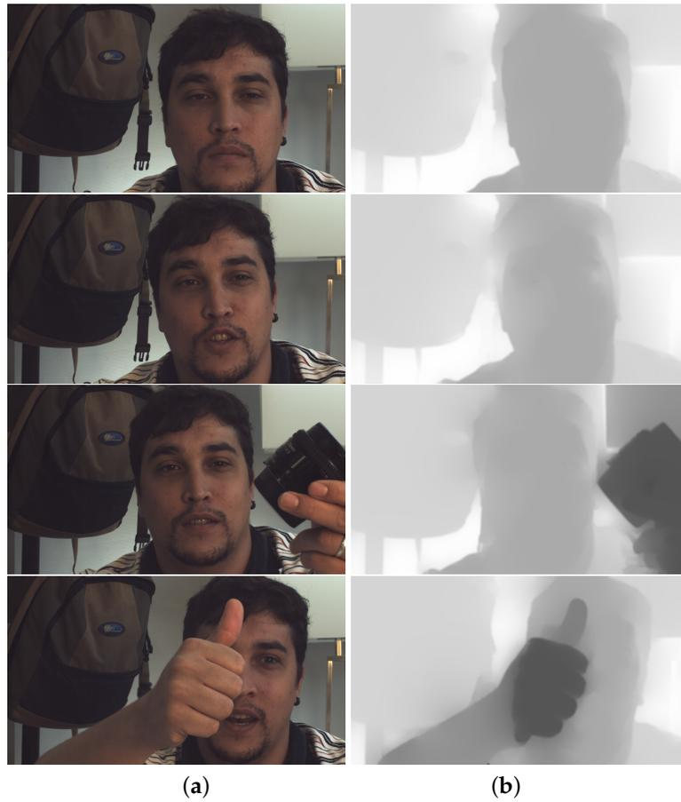
**Figure 9.** Frames selected from a video captured with the presented setup, in the left the all in focus image, and in the right the dense depth map. (a) AIF. (b) Depth map.
