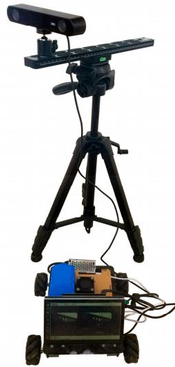
**Figure 12.** Experimental platform of the spatial location of binocular camera.
