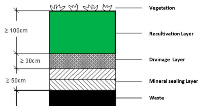
**Figure 1.** Different layers involved in landfill capping—Landfill Class I Germany (Adapted source: [30]).
