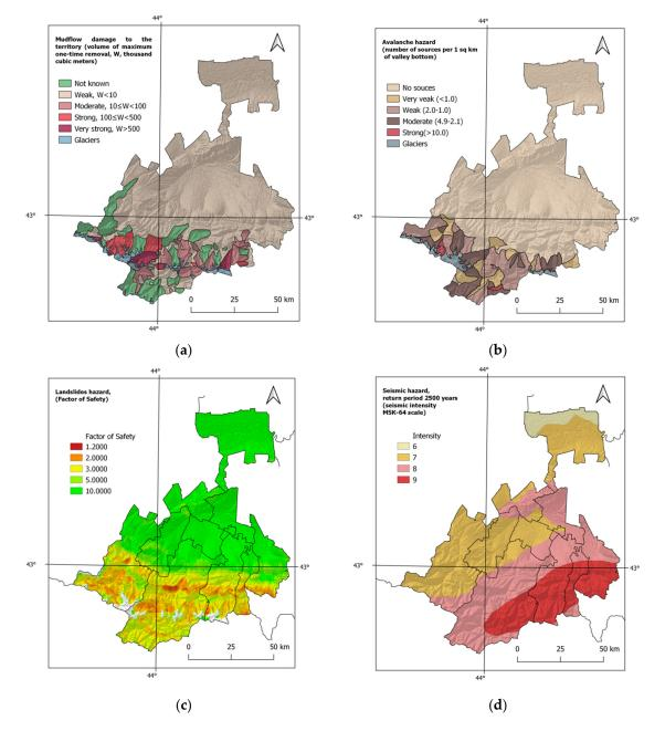
**Figure 4.** (a)Scheme of mudflow hazardous zones of North Ossetia-Alania; (b) scheme of avalanche hazard on the territory of North Ossetia-Alania [33]; (c) assessment of the potential landslide hazard of the territory of North Ossetia-Alania in the form of a safety factor F; (d) seismic hazard map of the territory of North Ossetia-Alania, intensity with 5% exceedance probability.
