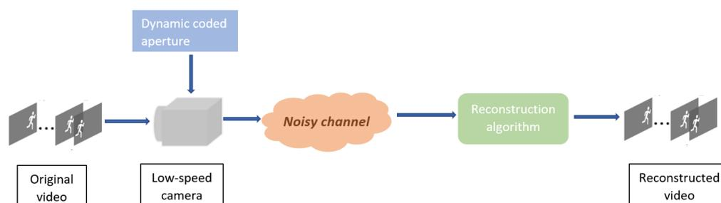
**Figure 2.** basic model of video compressive sensing.
