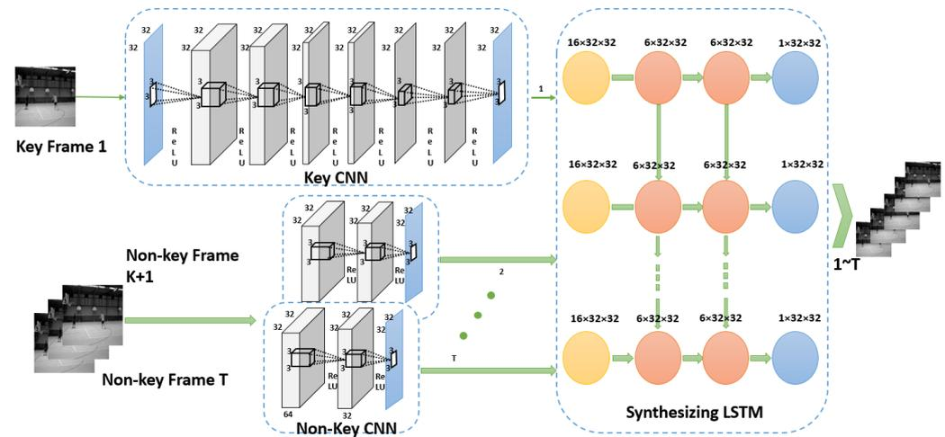
Figure 7. CSVideoNet Architecture.
