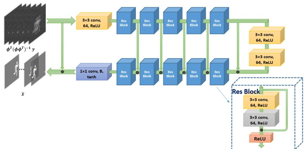
Figure 6. E2E-CNN Architecture.
