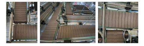
Figure 27. Perpendicular position between two conveyors.
