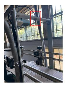
Figure 28. The installation position of proximity sensors on the sub-conveyors.
