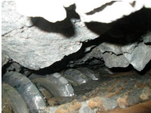
Figure 6. Disc cutter tools.
