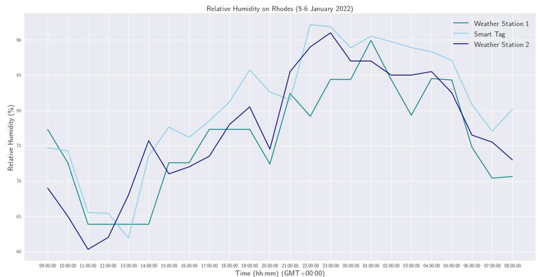
**Figure 15.** Relative Humidity on Rhodes at 5 January 2022 measured by a Smart Tag and two commercial weather stations.
