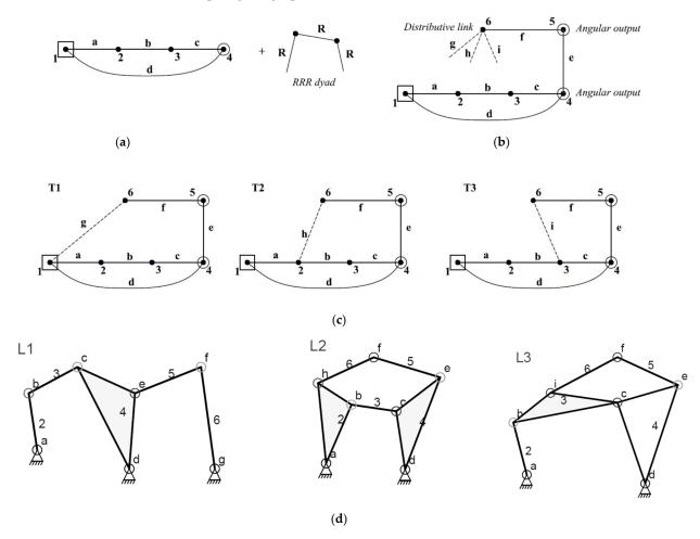
**Figure 4.** Generation of two angular output motions. (a) Initial linkage having one output; (b) new output 'link-5' is added; (c) available topologies having two outputs; (d) corresponding linkage diagrams.
