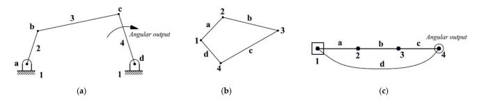
**Figure 1.** Representation of a four-bar mechanism. (a) Kinematic structure of a four-bar mechanism; (b) graph representation of a four-bar mechanism; (c) modified graph representation of a four-bar mechanism.
