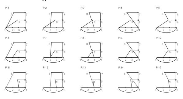
**Figure A1.** A complete set of eight-bar linkage topologies with three angular outputs using parallel connection.
