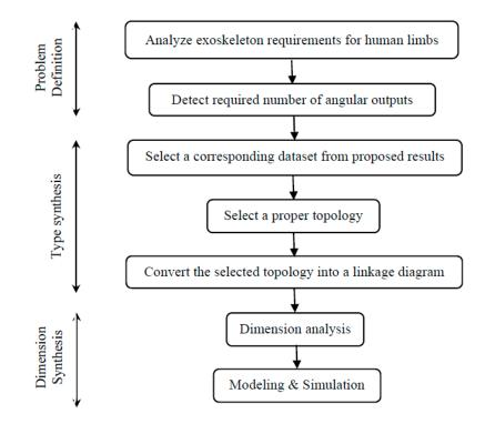
Figure 9. Exoskeleton design procedures.
