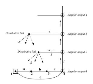
Figure 2. Generation of newer angular outputs using parallel connection.
