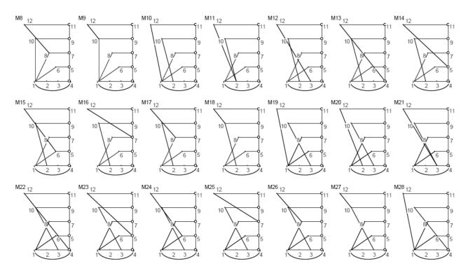
Figure A4. Some of the twelve-bar linkage topologies with five angular outputs using parallel connection.
