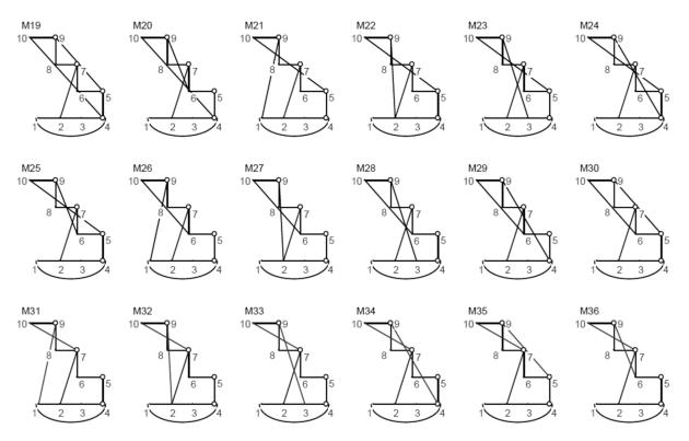
Figure A3. Some of ten-bar linkage topologies with four angular outputs using series connection.
