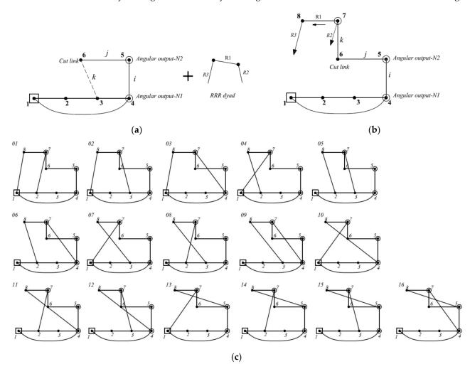
**Figure 6.** Generation of three angular outputs using series connection. (**a**) Initial graphical topology having two outputs; links: 4, 5; (**b**) new output 'link-7' is added; (**c**) all available topologies of three outputs with series connection.
