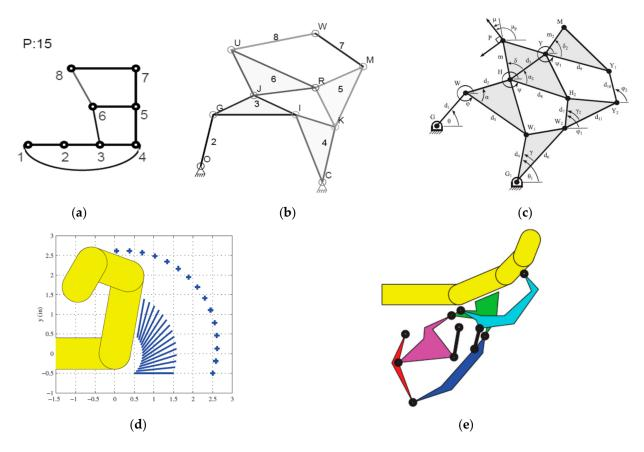
**Figure 7.** Using eight-bar linkage as exoskeleton for finger rehabilitation. (**a**) Selected graph from presented database; (**b**) corresponding linkage diagram; (**c**) equivalent exoskeleton linkage introduced by [21]; (**d**) desired motion for finger introduced by [21]; (**e**) resulting eight-bar linkage introduced by [21].
