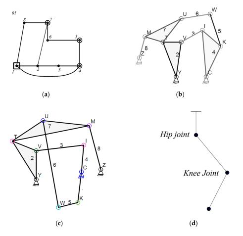
**Figure 8.** Using eight-bar linkage as exoskeleton for leg rehabilitation. (**a**) Selected graph from presented database; (**b**) corresponding linkage diagram; (**c**) equivalent exoskeleton linkage; (**d**) Lower limb joints.
