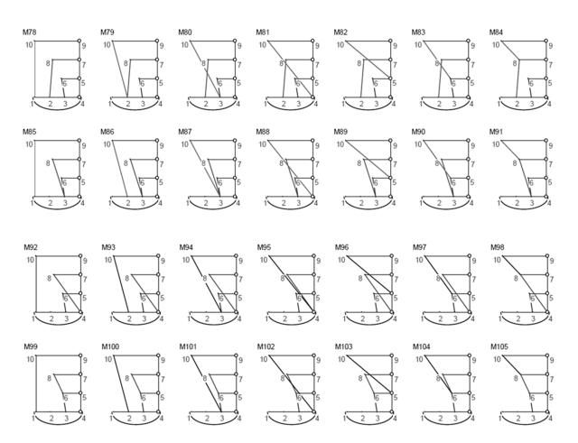
Figure A2. A complete set of ten-bar linkage topologies with four angular outputs using parallel connection.
