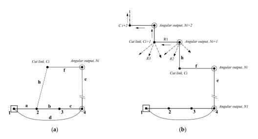
**Figure 3.** Generation of angular outputs using series connection method. (**a**) Initial topology with Ni outputs; (**b**) adding newer angular outputs and cut links.
