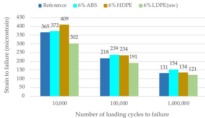
**Figure 11.** Comparison of tensile strain at 10,000, 100,000, and 1 million loading cycles used as a fatigue resistance indicator at 20 °C.
