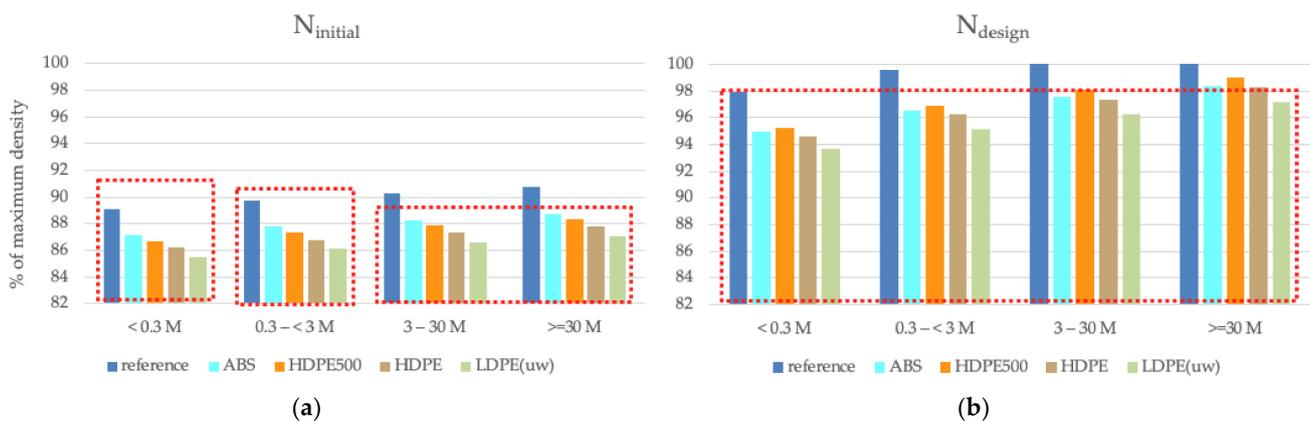
Figure 15. Comparison of the workability measured in gyratory compaction tests with the SUPERPAVE limits for (a)  $N_{initial}$  and (b)  $N_{design}$ .
