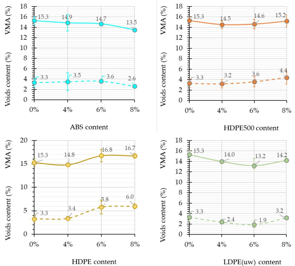
Figure 6. Variation of volumetric properties with the plastic waste content.
