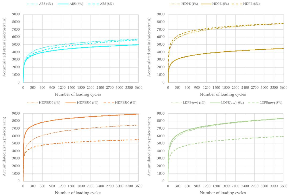
**Figure 13.** Influence of the plastic waste content on the accumulated permanent deformation measured in cyclic compression tests at 60 °C for the four types of plastic waste used.
