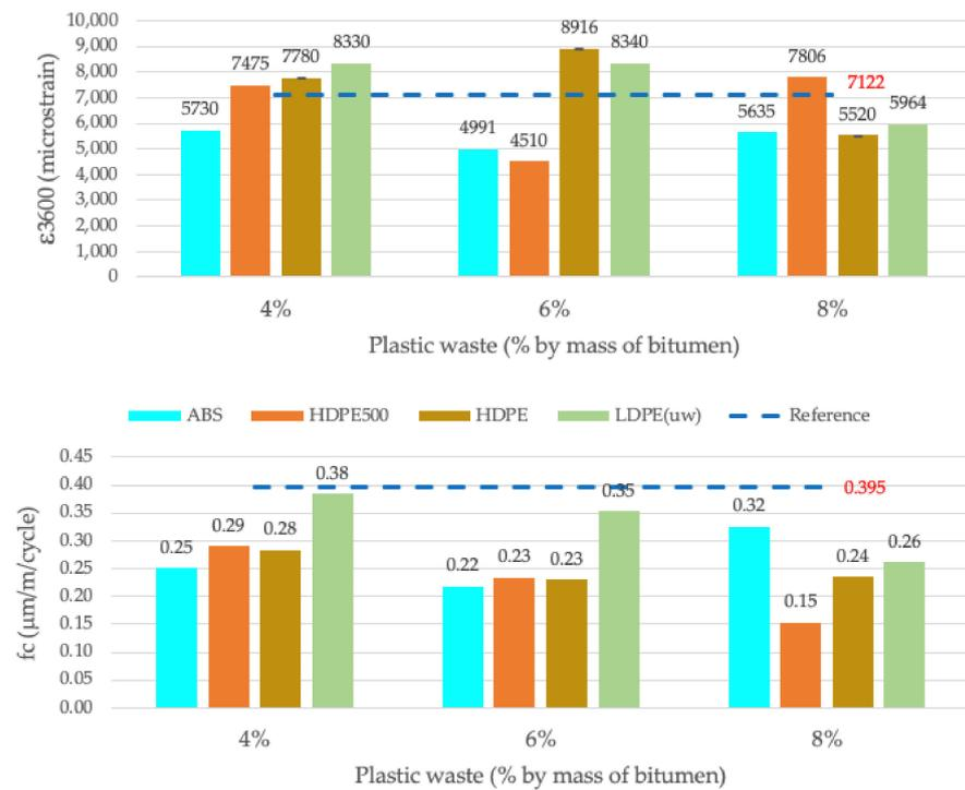
Figure 14. Results for the accumulated strain ( $\epsilon_{3600}$ ) and creep rate ( $f_c$ ).
