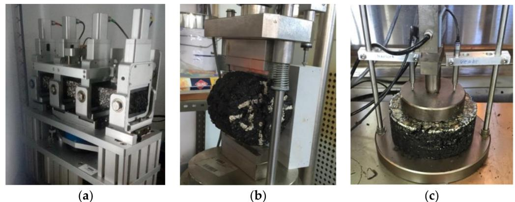
**Figure 5.** Mechanical performance tests: (a) four-point bending test; (b) indirect tensile strength test; and (c) cyclic compression test.
