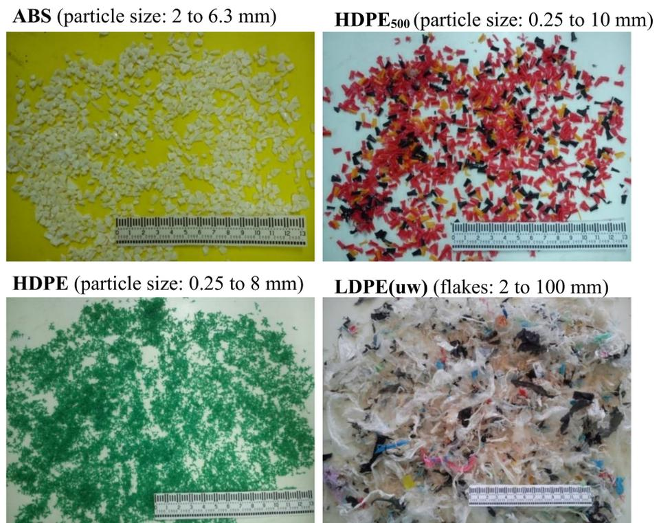
**Figure 2.** Types of plastic waste used as polymers in the studied asphalt mixtures in the present study.
