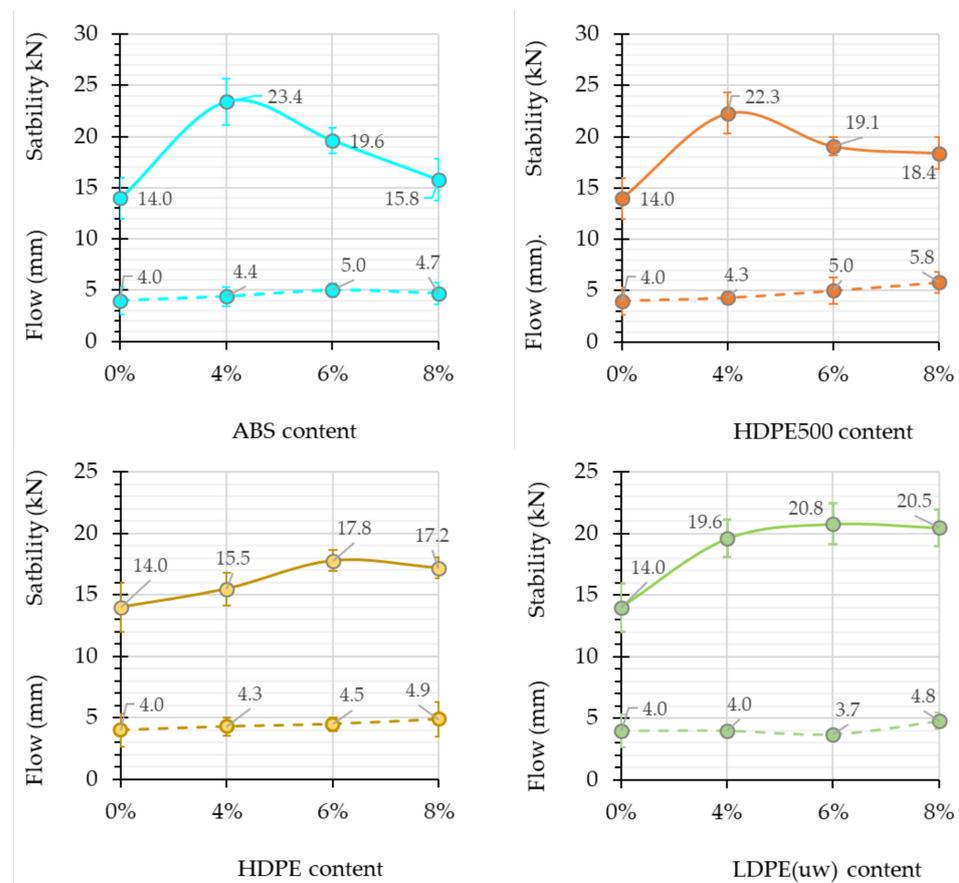
Figure 7. Marshall stability and flow as a function of plastic waste content.
