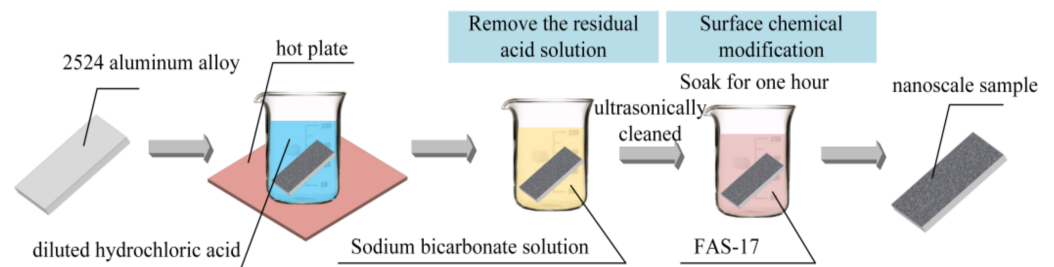
Figure 1. The wet etching procedure and key steps.
