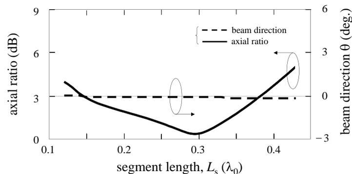
**Figure 5.** Simulated beam direction and axial ratio versus segment length  $L_s$  for a branched line antenna with  $N = 12$ .
