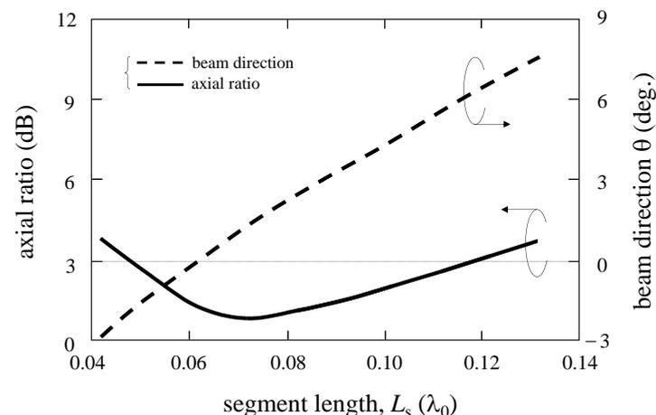
**Figure 3.** Simulated beam direction and axial ratio versus segment length  $L_s$  for a bent line antenna with  $N = 12$ .
