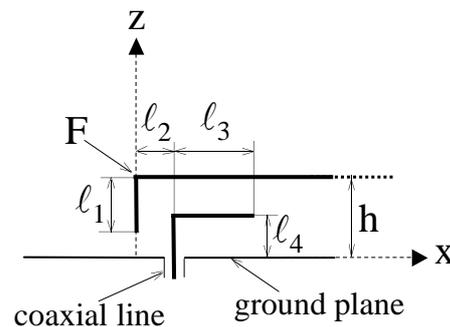
Figure 7. Electromagnetic-coupling feed for impedance matching.
