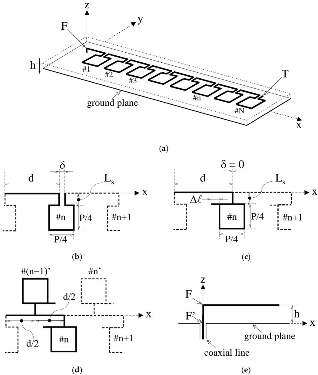
**Figure 1.** Antenna configurations: (a) perspective view; (b) bent line antenna having loops with a gap  $\delta$ ; (c) branched line antenna having loops without a gap ( $\delta = 0$ ); (d) modified branched line antenna with additional loops  $\#n'$ ; (e) side view with a vertical wire  $F-F'$ .
