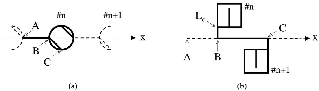
**Figure 2.** Antenna configurations in [3,7]: (a) bent line antenna [3]; (b) branched line antenna [7].
