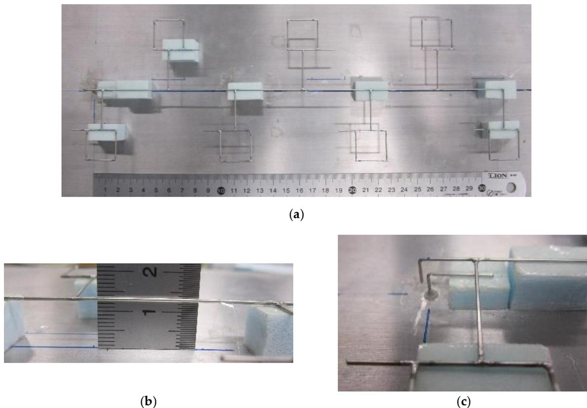
**Figure 10.** Prototype of a modified branched line antenna with  $N = 4$ : (a) top view; (b) side view; (c) perspective view of an electromagnetic-coupling feed.
