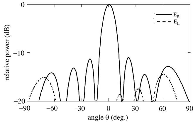
Figure 6. Simulated radiation pattern in  $\phi = 0^\circ$  plane for a branched line antenna with  $N = 4$ .
