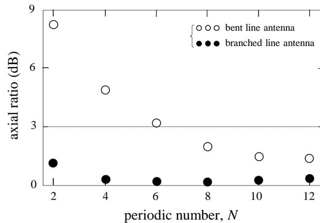
**Figure 4.** Simulated axial ratio versus periodic number  $N$ .
