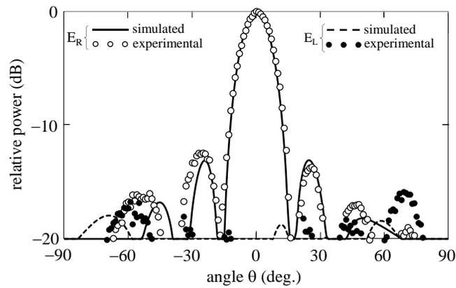
Figure 8. Radiation pattern in  $\phi = 0^\circ$  plane for a modified branched line antenna with  $N = 4$ .
