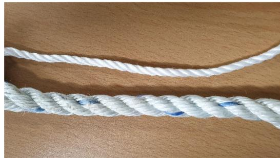
**Figure 9.** Polypropylene ropes for the cutting test in the laboratory-scale.
