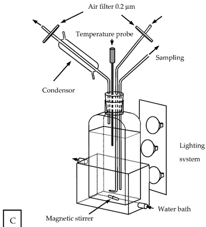
**Figure 1.** Experimental device used for the *L. indica* PCC8005 cultivation. (A) Cultures with magnetic field application through coils and (B) cultures control without MF application but in the same temperature, luminosity and aeration conditions. (1) Coils with 400 turns used to generate the MF, (2) illumination provided by 3 halogen lamps and (3) 600 mL photobioreactors. (C) Scheme of the experimental devices (control).
