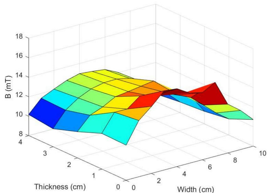
**Figure 3.** MF intensity mapping at a 7 cm height (middle of the culture vessel). Raw values are available in the Supplementary Materials.
