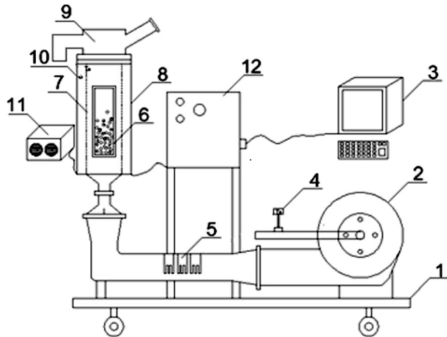
**Figure 2.** Laboratory stand for spouted bed-microwave drying (MP20): 1-rack; 2-fan; 3-computer; 4-temperature sensor; 5-electric heaters; 6-spouted bed; 7-drying chamber; 8-outside shield stopping microwaves; 9-cover; 10-temperature and pressure sensor; 11-magnetrons [40].
