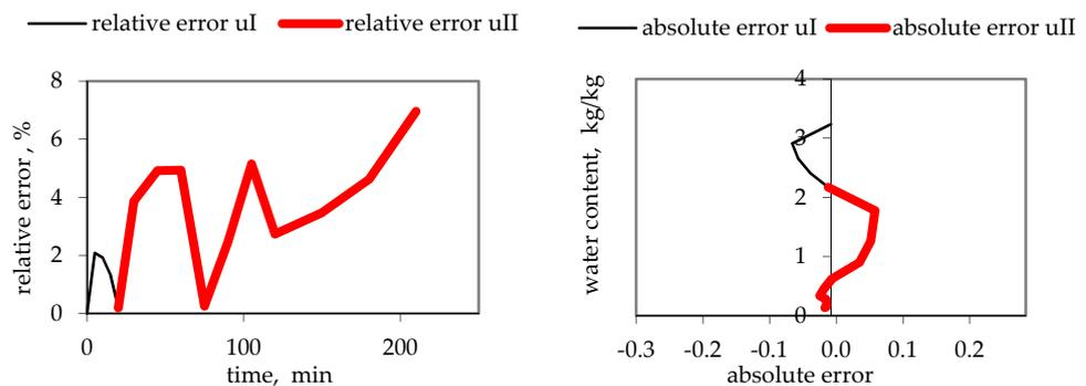
**Figure 4.** Relative and absolute errors for modeling of water content changes in the process of drying apple pomace in forced convection at 40 °C.
