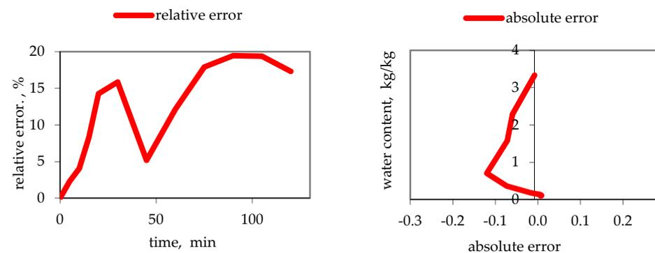
**Figure 12.** Relative and absolute errors for Page modeling of water content changes in the process of drying apple pomace in forced convection at 80 °C.
