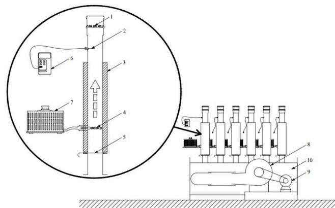
**Figure 1.** Convective drier scheme: 1-material basket; 2-sensor; 3-air supply duct; 4-heating element; 5-regulating valve; 6-heat recorder; 7-autotransformer; 8-fan; 9-engine; 10-expansion tank [39].
