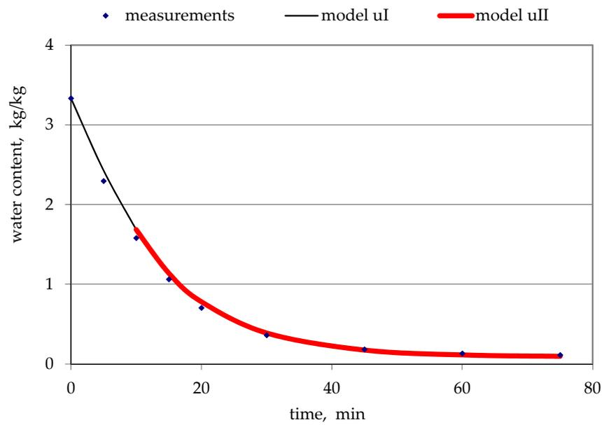
**Figure 5.** The graph of models for the changes in water content during the process of drying apple pomace in forced convection at 80 °C.
