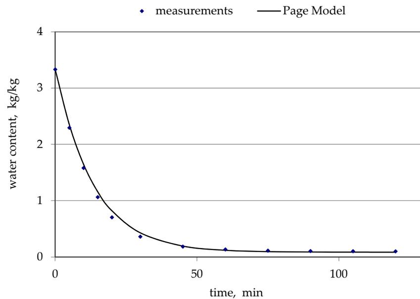
**Figure 11.** The Page model of water content changes in the process of drying apple pomace in forced convection at 80 °C.
