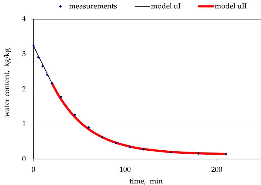
**Figure 3.** Modeling changes of water content in the process of drying apple pomace in forced convection at 40 °C.
