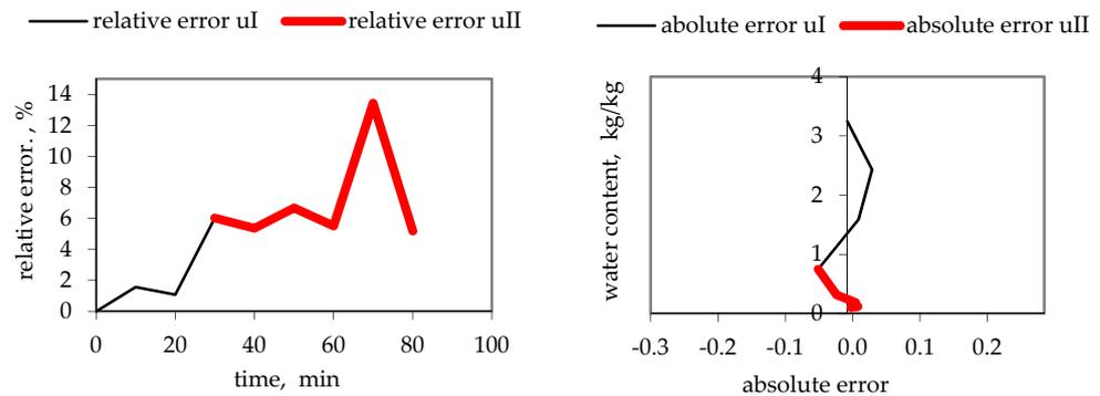
**Figure 8.** Relative and absolute errors for modeling of water content changes in the process of drying apple pomace in forced convection at 60 °C with microwave support (240 W).
