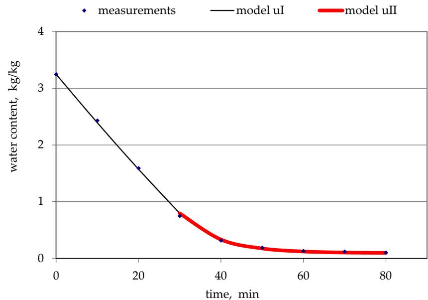
**Figure 7.** The graph of models of water content changes in the process of drying apple pomace in forced convection at 60 °C with microwave support (240 W).
