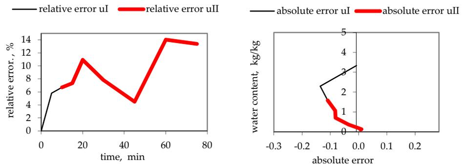
**Figure 6.** Relative and absolute errors for modeling of water content changes in the process of drying apple pomace in forced convection at 80 °C.
