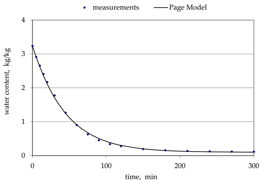
**Figure 9.** The Page model of water content changes in the process of drying apple pomace in forced convection at 40 °C.
