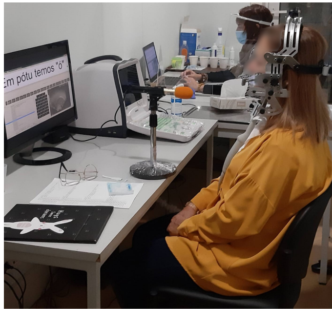
Figure 1. Experimental setup for recording ultrasound: the participant is seated in front of a microphone, wearing a stabilization helmet to keep the ultrasound probe positioned below the chin throughout the experiment. The prompts are presented on a computer monitor.
