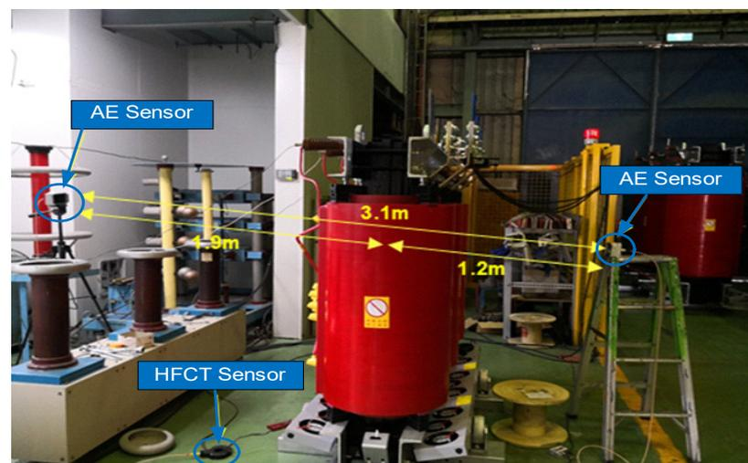
**Figure 12.** Installation of AE sensor and HFCT sensor without housing of transformer.
