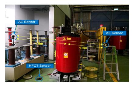
Figure 12. Installation of AE sensor and HFCT sensor without housing of transformer.
