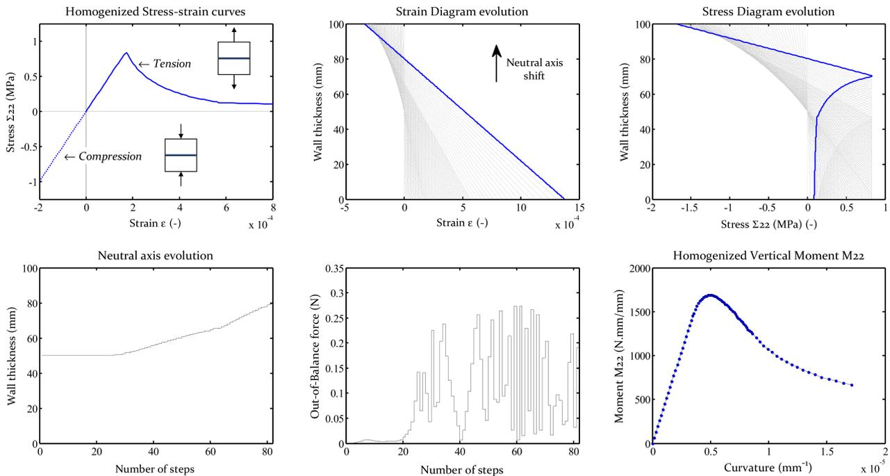
**Figure 8.** Procedure for integrating the homogenised vertical stress–strain curves on the masonry thickness aiming to obtain the homogenised vertical bending moment curve for the benchmark test.
