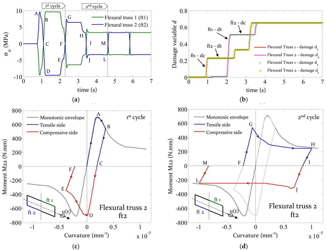
**Figure 11.** Bi-directional cyclic loading. (a) Cauchy stress  $\sigma_{11}$  for flexural trusses. (b) Evolution of the damage parameter,  $d$ , for the flexural trusses. (c) Vertical bending moment–curvature (first cycle). (d) Vertical bending moment–curvature (second cycle).
