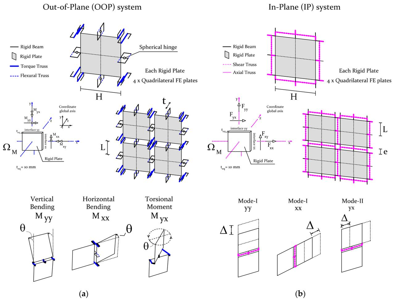
Figure 1. Macro-unit cell and kinematics of the macro-element. (a) Out-of-plane. (b) In-plane.
