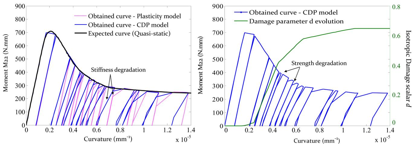
**Figure 10.** Uni-directional cyclic behaviour (Note: only the positive moments are plotted, i.e., the part of the unloading branch for negative bending moments has been disregarded for the sake of readiness).
