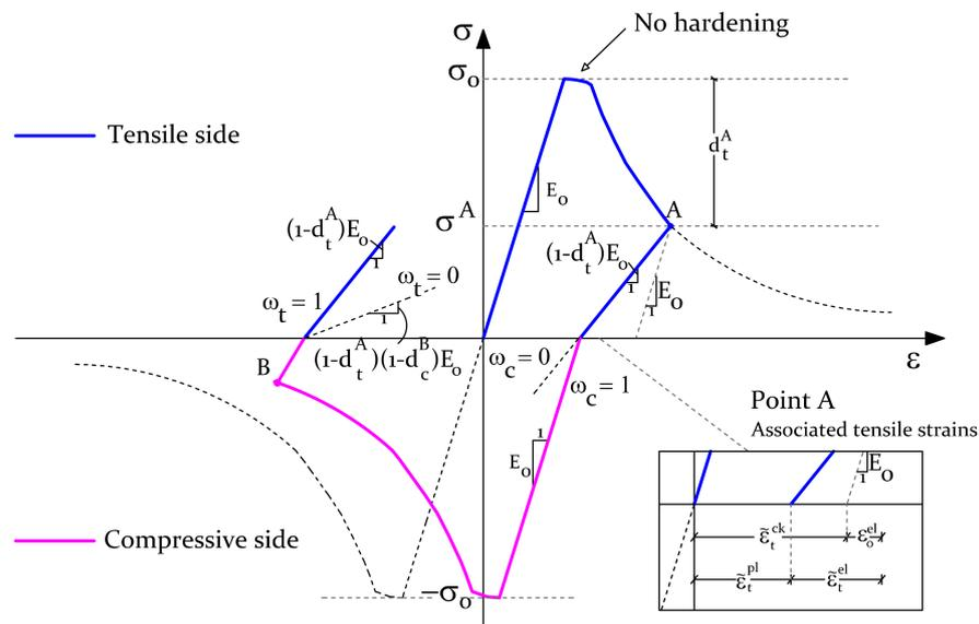
**Figure 4.** Hysteretic curve adopted for the out-of-plane trusses (note: for the in-plane truss beams, the tensile and compressive behaviours can have different shapes that stem from material characterisation).
