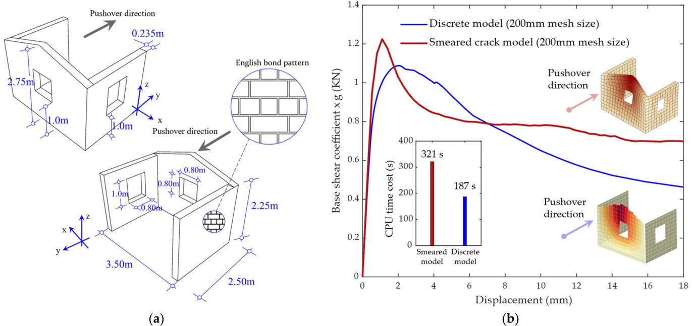
**Figure 12.** Capacity (pushover) curve and required CPU time for the LNEC house benchmark: comparison between the macro-element (discrete) model and smeared crack model. (a) Geometry of the LNEC brick house. (b) Capacity curves and required CPU time.
