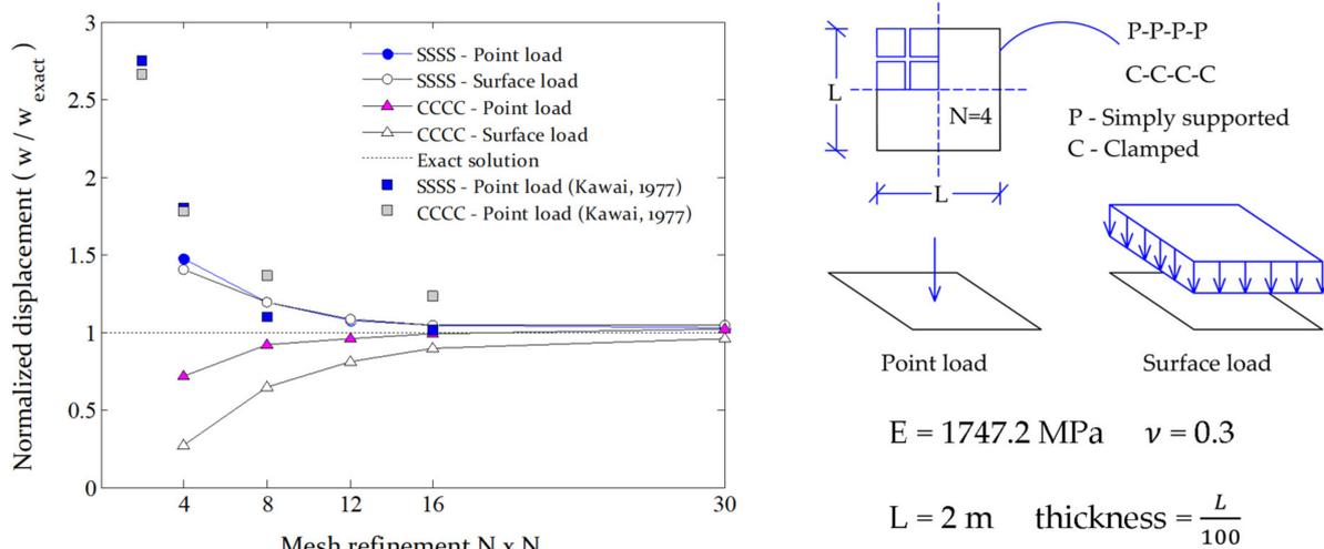
Figure 5. Convergence study conducted for a squared plate test.
