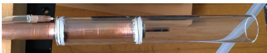
**Figure 2.** Image of the quartz channel for particle combustion.
