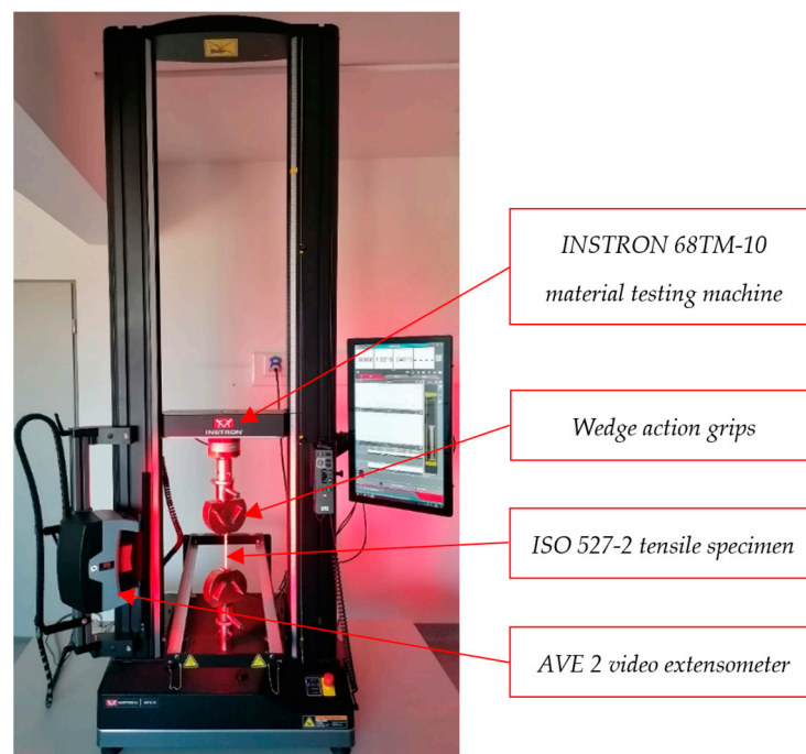
Figure 4. Testing setup for tensile testing.
