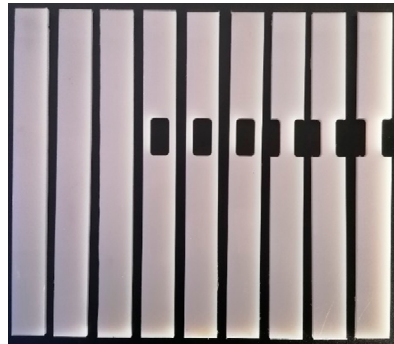
Figure 3. Manufactured specimens for the material model validation.
