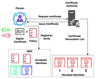
Figure 3. Identity certifications issuing and membership service provider verification.
