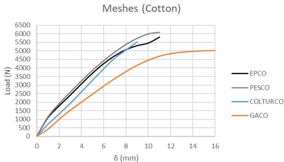
Figure 7. Load–Extensometer curves for cotton meshes.
