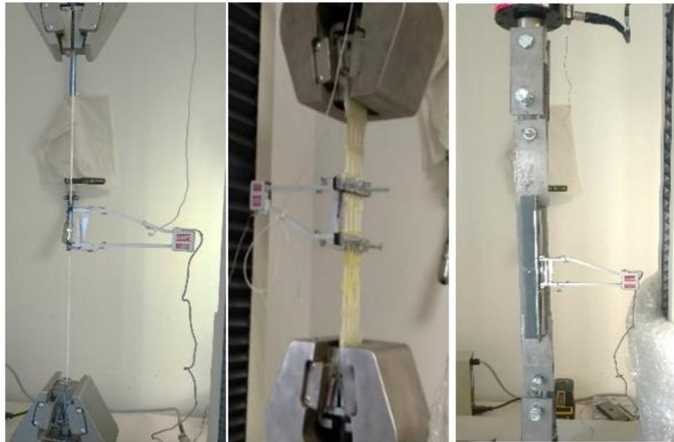
**Figure 3.** Tensile test setup: yarns (left), meshes (middle), FRCM (right).
