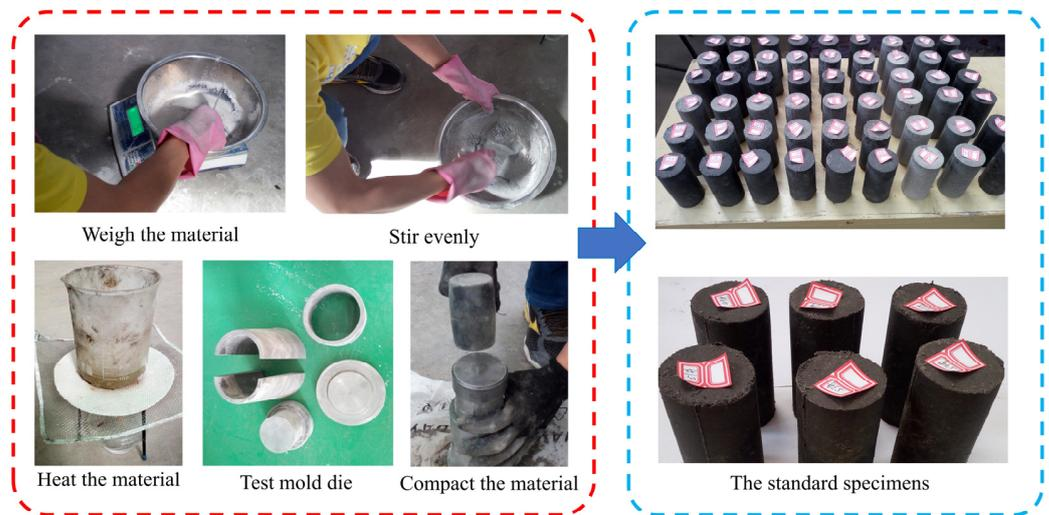
Figure 2. Similar material specimens-making process.
