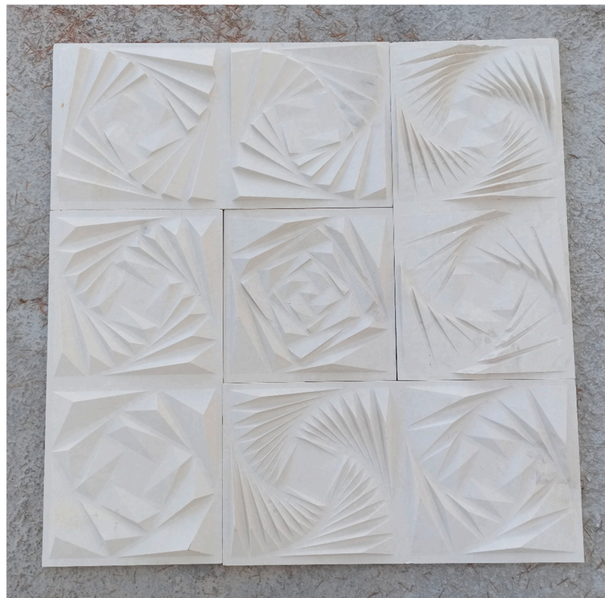
Figure 18. The result, generated with proposed method by applying different transformation rules defined with corner-weight , median-weight , height , and rotation parameters at each iteration ( center ) and the results generated by applying same transformation rules at each iteration ( others ).
