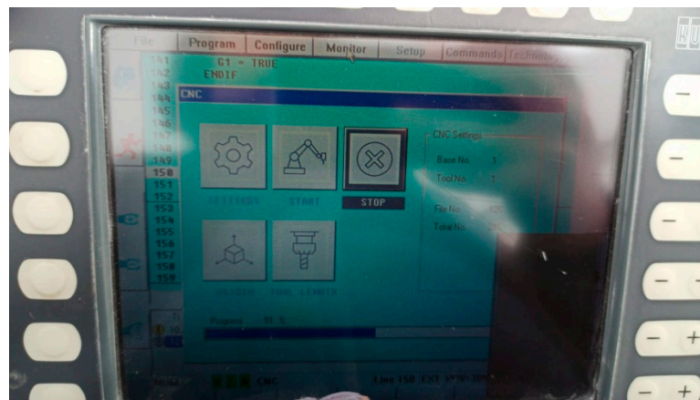
Figure 9. TCP Socket Server software screenshot on Kuka Control Robot Unit (VKRC2).
