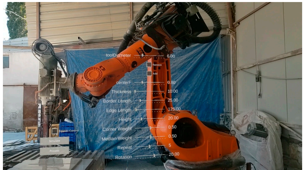
Figure 15. The user can access and change the parametric-design and robotic-fabrication parameters using the mixed-reality device.
