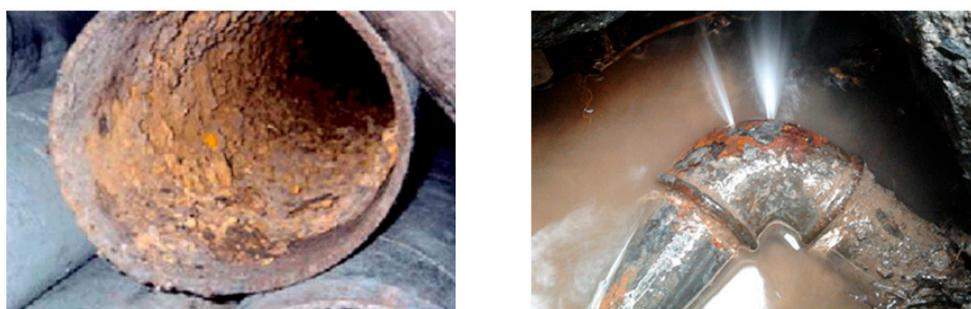
**Figure 2.** Pipeline corrosion and leakage diagram.
