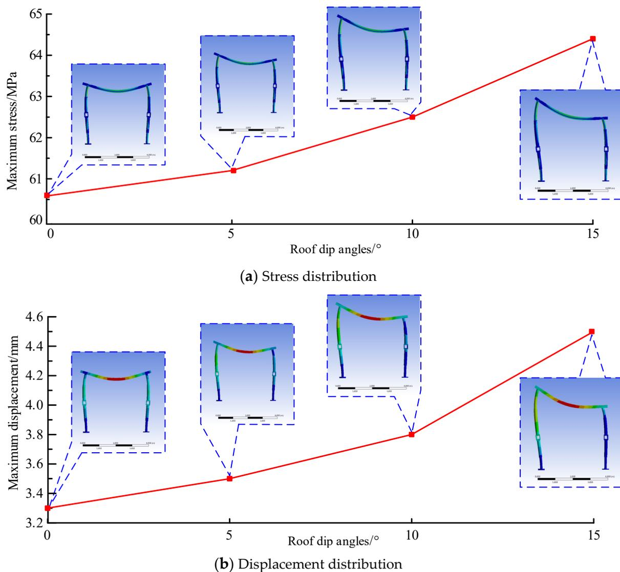
**Figure 7.** (a) Stress and (b) displacement distributions of the advance support under different roof-dip angles.
