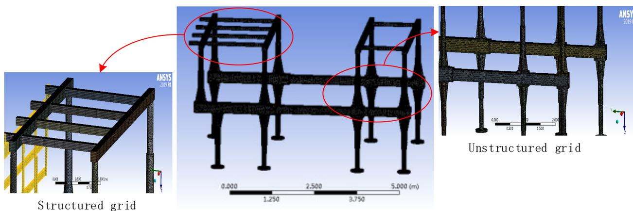
**Figure 4.** Overall finite element model of the advance support.
