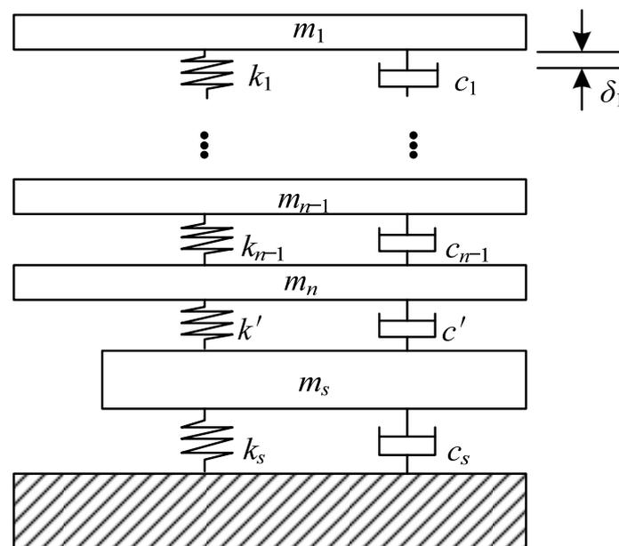
Figure 3. Simplified two-dimensional graph of the dynamic model of coupling between the advance support and the roof.
