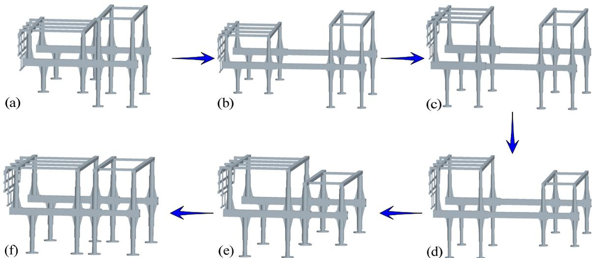
**Figure 2.** Working process of the new type of HAAS for fully mechanized roadways. (a) Support preparation; (b) Front support movement; (c) Front support expansion; (d) Rear support retracted; (e) Rear support movement; (f) Rear support expansion.
