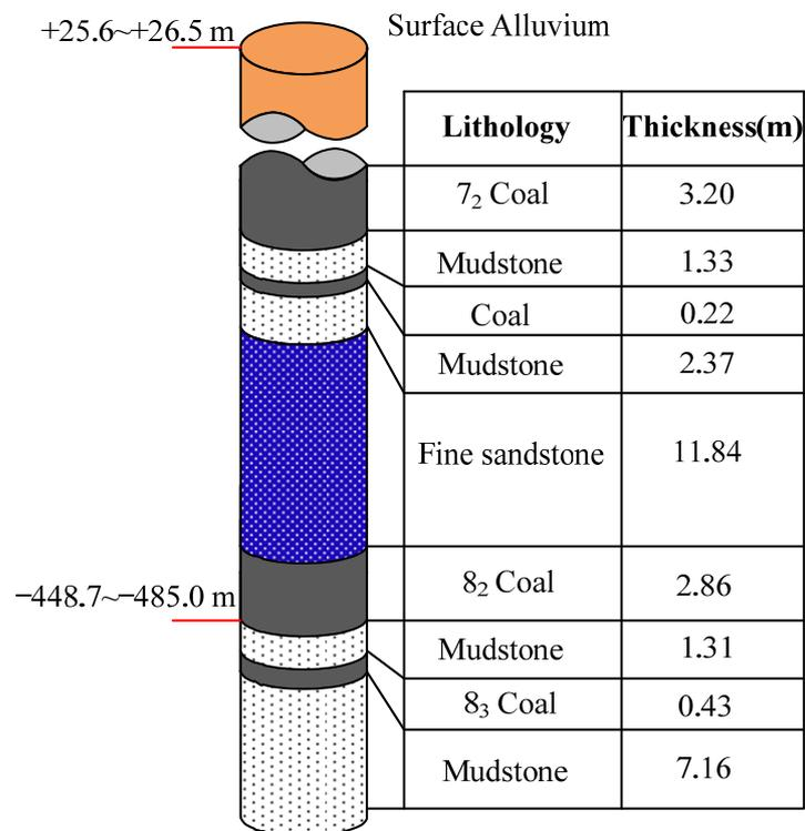
Figure 9. The stratigraphic column of the 8<sub>2</sub>24-machine roadway in the XT Coal Mine.
