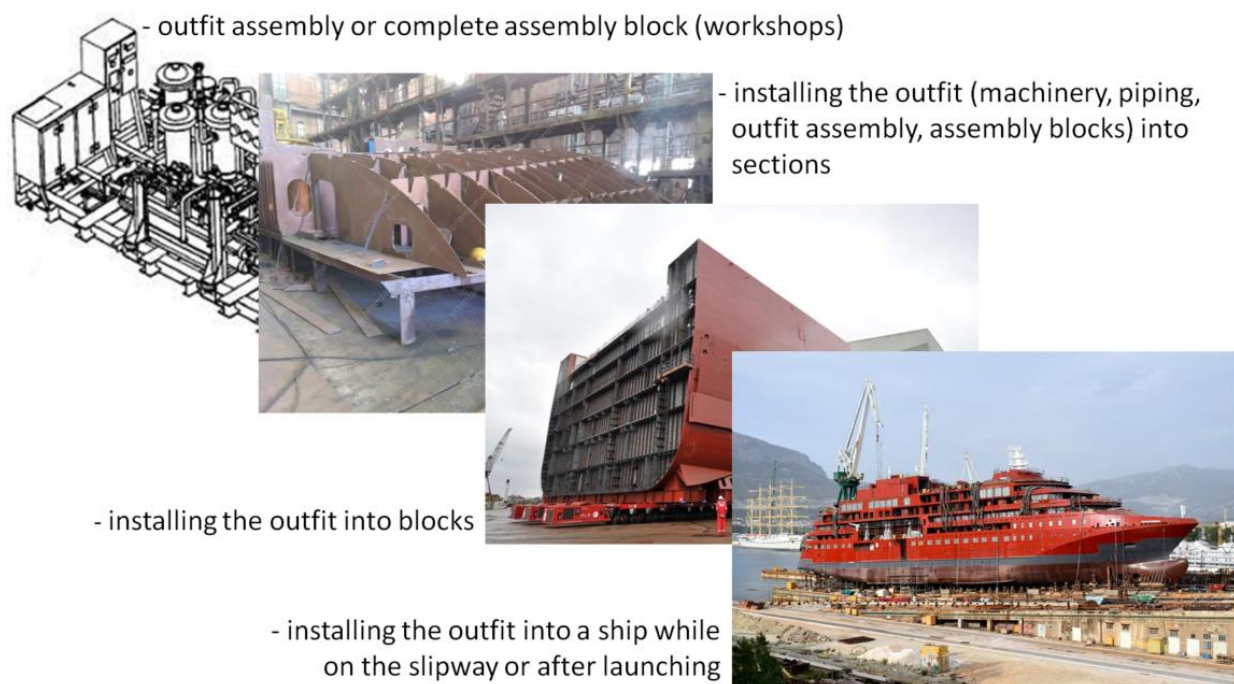
Figure 5. Advanced outfitting in relation to the shipbuilding stages.
