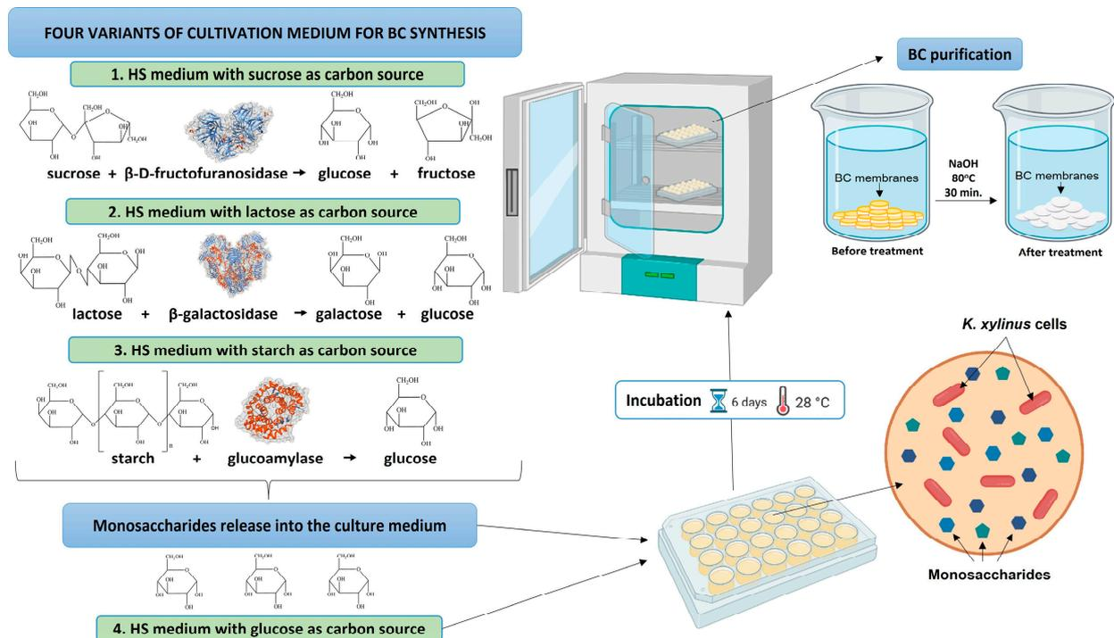
**Figure 1.** The scheme of the experimental *K. xylinus* cultivation process in the presence of a combination of oligo- and polysaccharides and specific enzymes.
