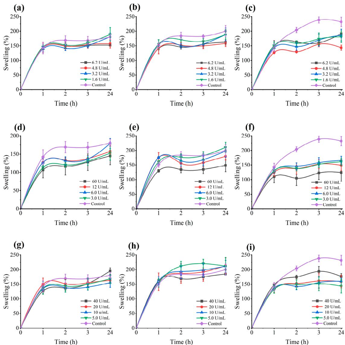
**Figure 6.** The influence of pH on the swelling ratio of BC obtained from analyses on cultivation media variant. The SR for BC obtained from the medium with sucrose and  $\beta$ -D-Fru at pH 4.0 (a), 5.0 (b) and 7.0 (c), lactose and  $\beta$ -Gal at pH 4.0 (d), 5.0 (e), and 7.0 (f); with starch and GLA at pH 4.0 (g), 5.0 (h), and 7.0 (i).
