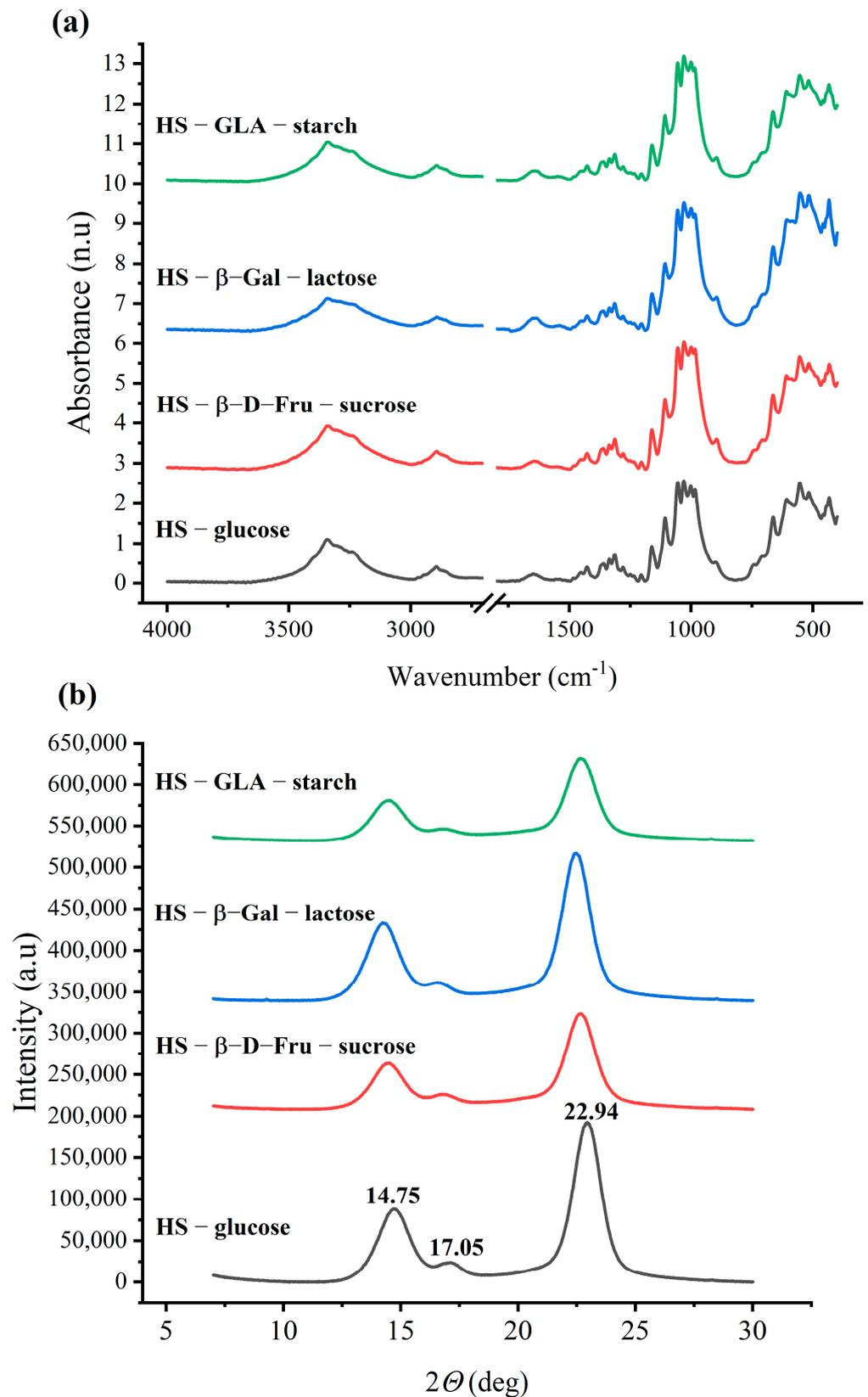
**Figure 4.** The representative ATR-FTIR spectra (a) and XRD diffractograms (b) of bacterial cellulose obtained from cultures with enzymatic conversion of sucrose, lactose, and starch to accessible carbon sources. The spectra from analysis BC samples obtained from modified media with the highest enzyme units amounts.
