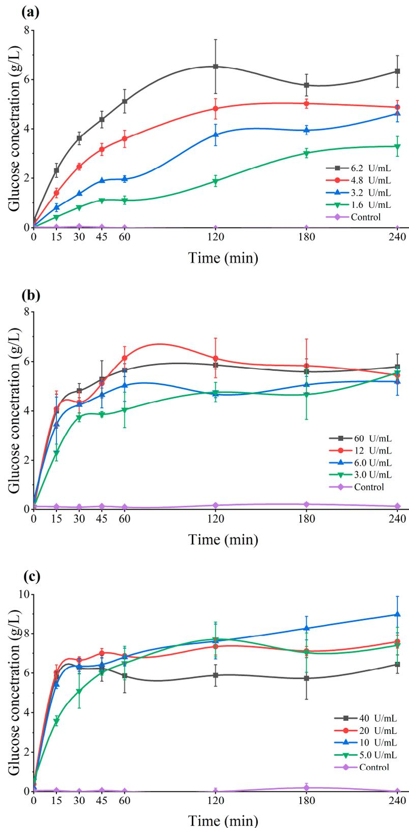
**Figure 2.** The effect of different amount units of  $\beta$ -D- Fru,  $\beta$ -Gal, and GLA on substrate conversion to simple sugars in HS medium with sucrose (a), lactose (b), and starch (c) as carbon sources.
