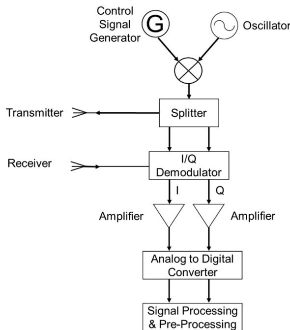
**Figure 3.** Architecture design of FMCW radar [21].
