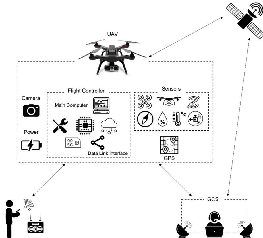
**Figure 1.** High-level architecture of a UAV.
