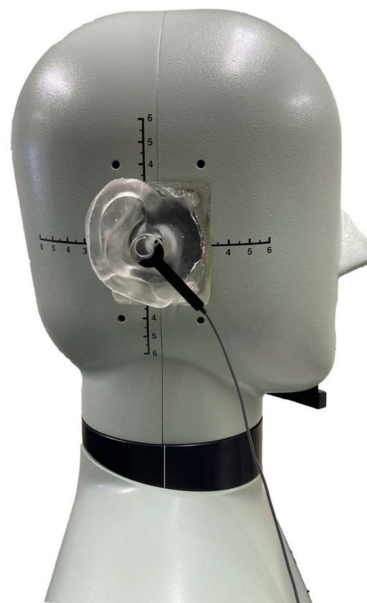
Figure 2. (a) Developed pinna simulators (A10, A20, and A40 from the left) and (b) embedded pinna simulator in the HATS and position of the cartilage conduction transducer at the entrance of the external auditory canal.
