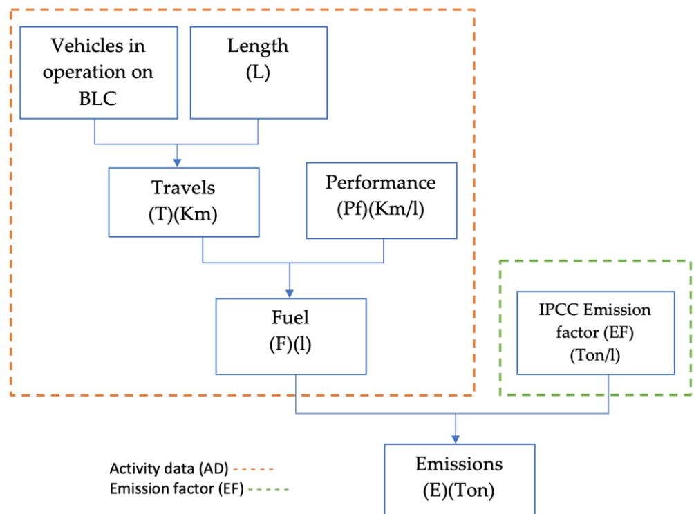
Figure 4. Emissions estimation model (own elaboration) based on IPCC [35].
