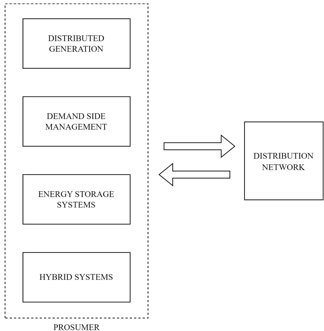
**Figure 1.** Prosumer configuration and interconnection with DNs.
