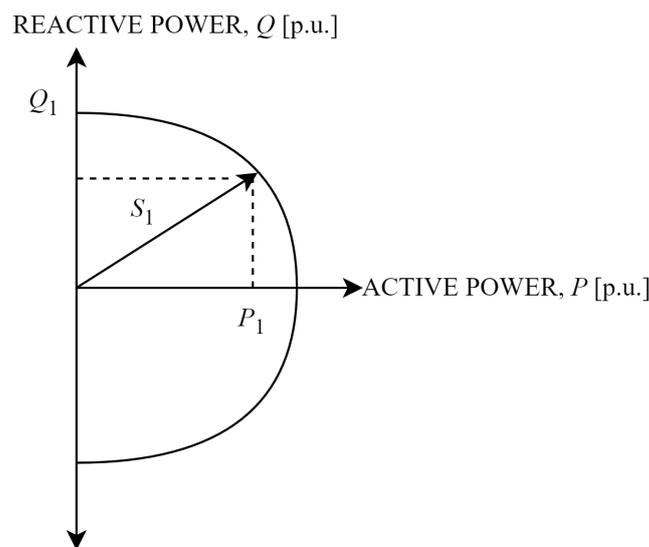
**Figure 3.** Power capability curve of PV inverter.
