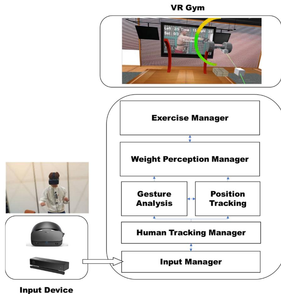
Figure 2. System architecture.
