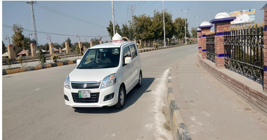
**Figure 2.** Instrumented test vehicle containing a roof-mounted antenna along with a PolARx5s multi-frequency and multi-constellation GNSS receiver as used for field experimentation and data acquisition.
