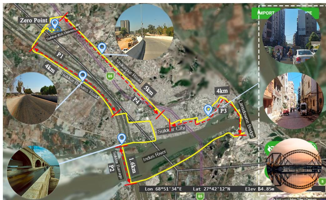
**Figure 1.** A 30 km long route covering the Sukkur city center and its surroundings used for field experimentation contain various operating environments, such as clear open-sky at the N-65 highway, semi-urban and dense urban areas with small lane widths, high-rise buildings, flyovers and bridges. The total route is divided into four distinct observation windows based on environment characteristics, and these are labeled as P1, P2, P3 and P4.
