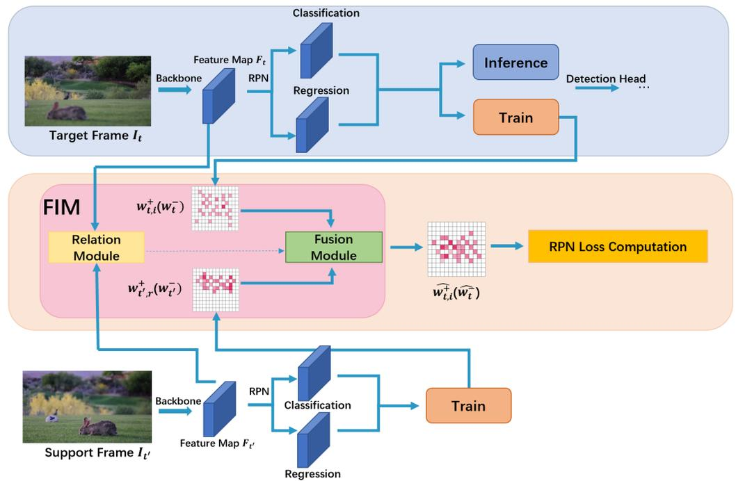
**Figure 2.** The architecture of our temporal guided label assignment (TGLA). The temporal-guided label assignment framework is presented by the upper blue box and the lower orange box, which denote forward propagation and loss computation separately. Note that the framework we mentioned below does not include feature instructing. Furthermore, we put forward an feature instructing module (FIM), which utilizes feature maps to guide the fusion of weight maps.
