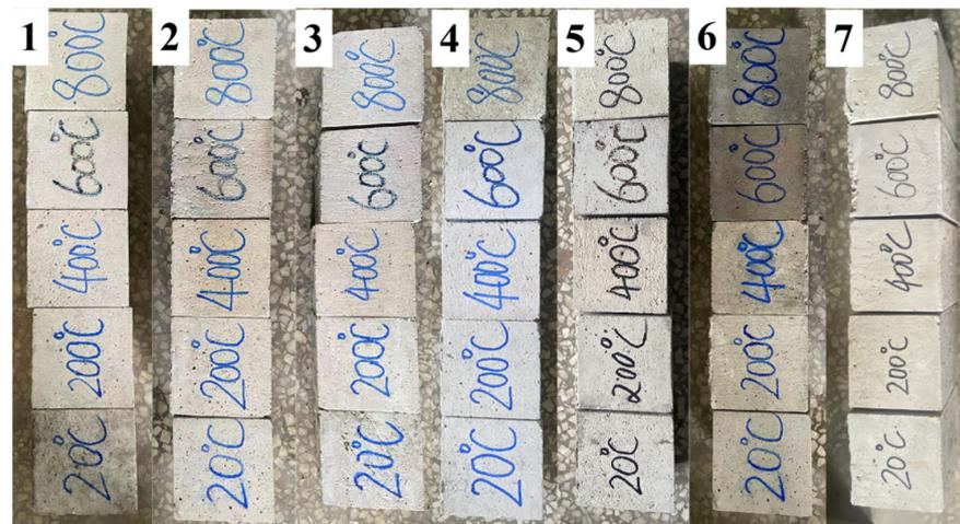
Figure 10. Appearance of concrete specimens before and after high-temperature exposures.
