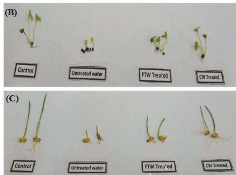
**Figure 9.** Bioassay to compare the treated water of CWs and FTWs: (A) visual comparison of turbidity level of contaminated water treated in CTWs and FTWs; (B) *Brassica napus* seed germination in treated water of CWs and FTWs; (C) *Triticum aestivum* seed germination in treated water of CWs and FTWs.
