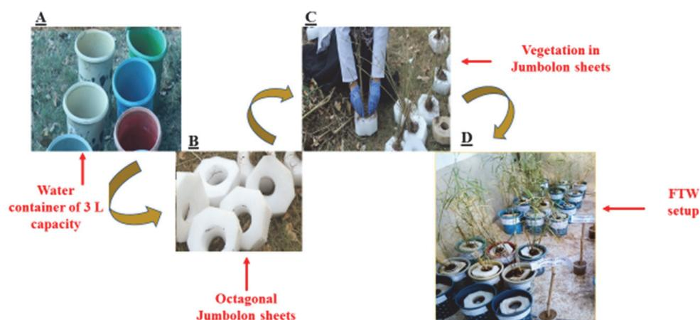
**Figure 1.** Development of floating treatment wetlands. Where, (A) shows the water containers, (B) shows octagonal jumbolon sheets, (C) shows the vegetation process, and (D) shows experimental setup.
