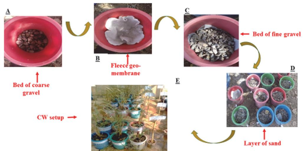
**Figure 3.** Development of constructed wetlands. Where, (A) shows the bed of coarse gravel, (B) shows fleece membrane, (C) shows bed of fine gravel, (D) shows layer of sand, and (E) shows experimental setup.
