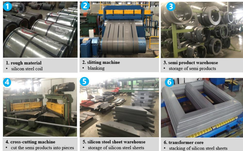
**Figure 1.** Production process of a transformer core.
