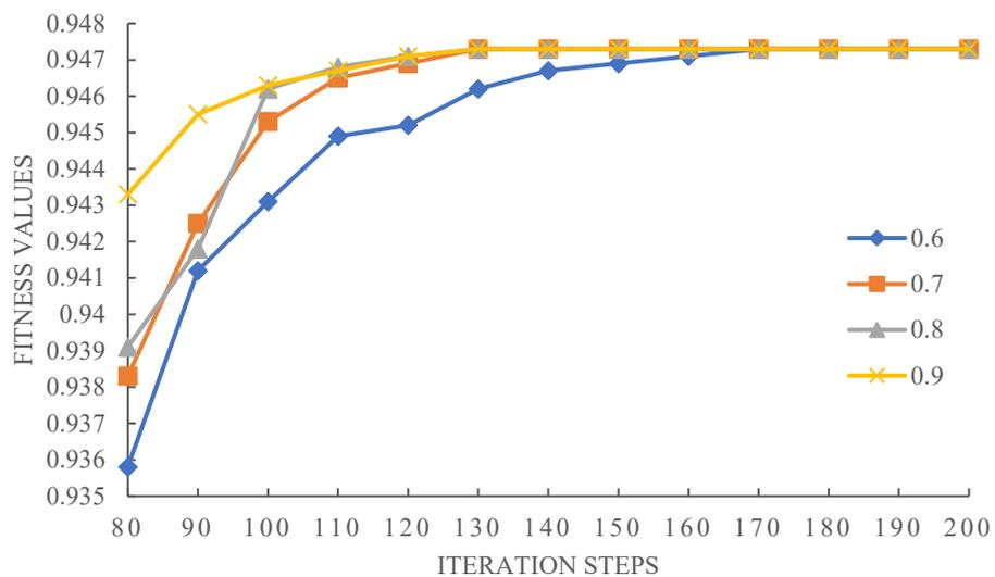
Figure 5. Relationship between the fitness value and iteration steps when  $P_{cross}$  varied.
