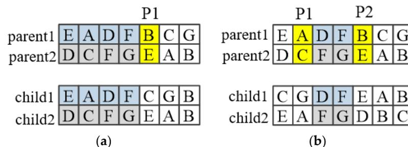
Figure 3. Crossover methods. (a) single-point crossover. (b) double-point crossover.
