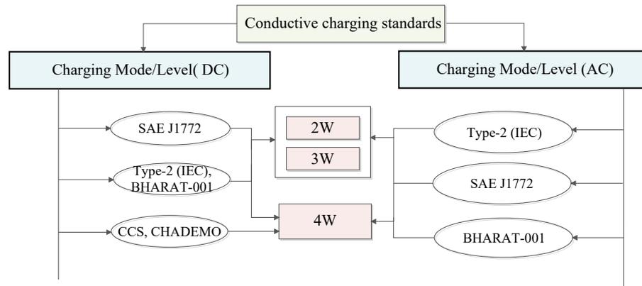
Figure 6. Taxonomy of conductive charging standards based on the type of EV.
