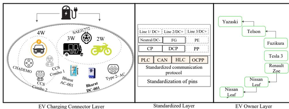
Figure 9. The proposed EV charging station standardization architecture.
