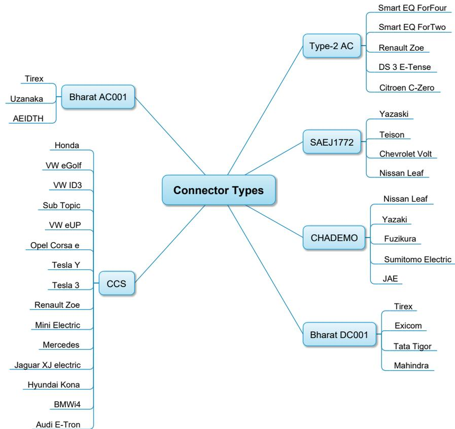
Figure 5. Taxonomy of charging connectors based on the manufacturers.
