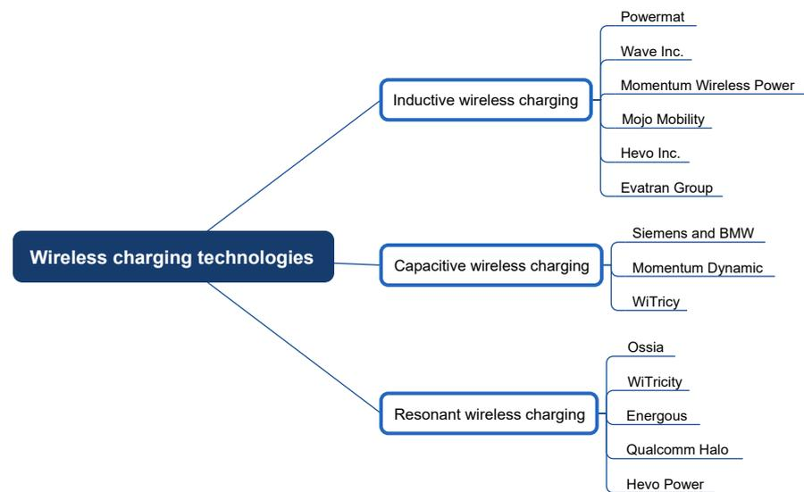
**Figure 8.** Taxonomy of wireless technologies based on the manufacturer.
