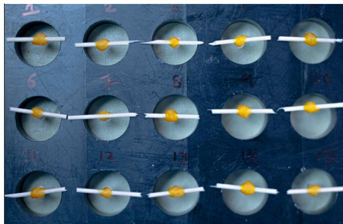
**Figure 1.** Teeth were mounted in acrylic-resin blocks using a test mount former.
