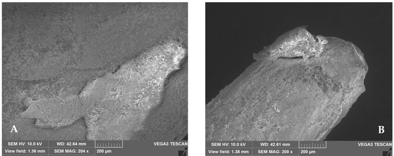
**Figure 12.** Scanning-electron-microscope image of (A) Sectioned root canal, and (B) displaced post, at 200× magnification, showing cohesive failure mode in Group 4 (CMZPCs) sample at root/post interface.
