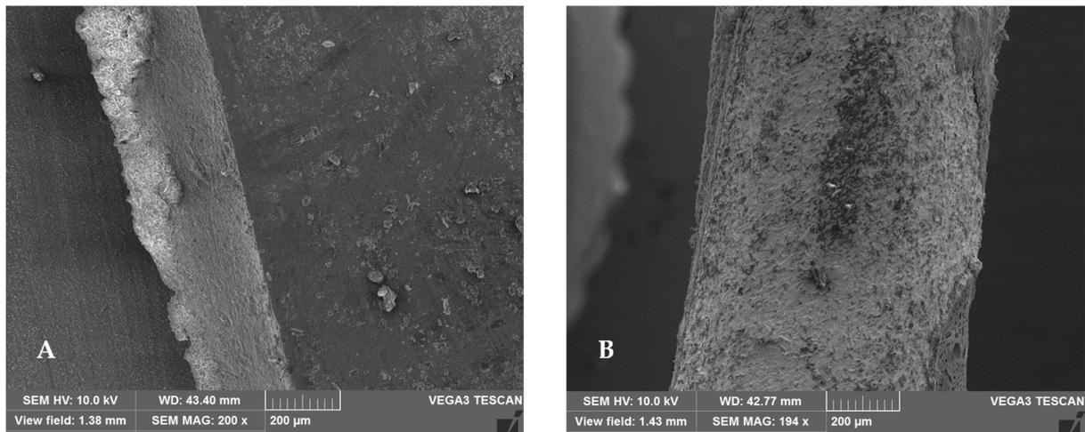
**Figure 9.** Scanning-electron-microscope image of (A) Sectioned root canal, and (B) displaced post, at 200× magnification, showing cohesive failure mode in Group 1 (CCNPPCs) sample at root/post interface.
