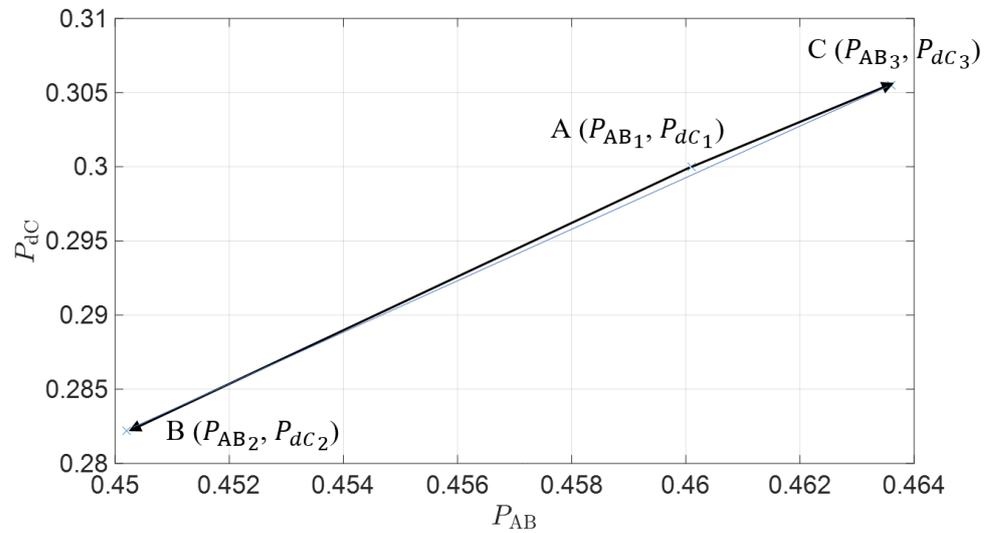
Figure 2.  $P_{AB} - P_{dC}$  diagram of N-KZFS11, N-SF66, and N-PK52A.
