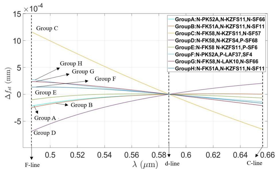
**Figure 8.** Optimized real lateral chromatic aberration curve for the eight triplet lens groups selected by the illustration method.
