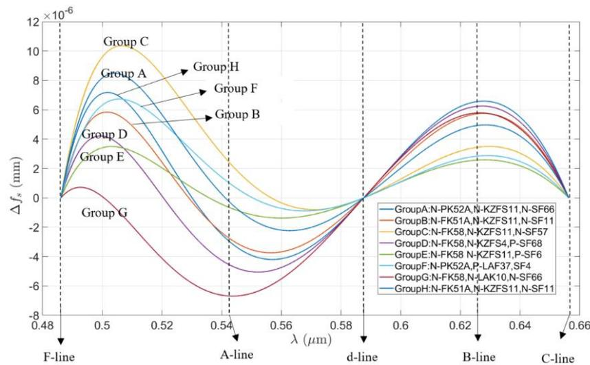
Figure 5. Chromatic aberration curves of the eight triplet lens combinations selected by the illustration method.
