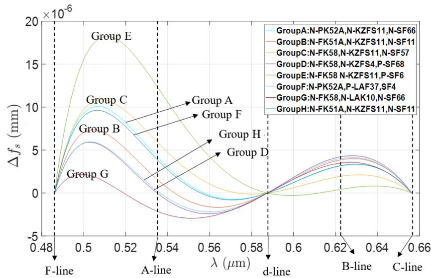
**Figure 7.** Real longitudinal chromatic aberration curve optimized for the eight triplet lens groups selected by the illustration method.
