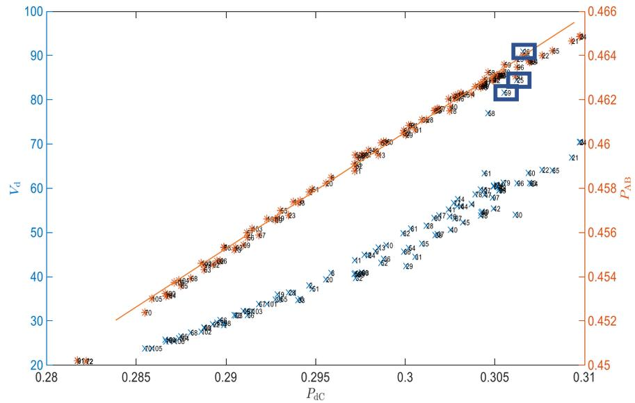
Figure 3.  $V_d - P_{dC}$  and  $P_{AB} - P_{dC}$  diagrams for the 106 SCHOTT glass materials.
